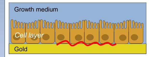
Surface plasmon senses: •cell refractive index •cell-substrate adhesion
