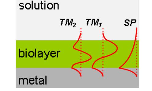
Surface plasmon (SP) senses the part of the layer in contact with substrate.
