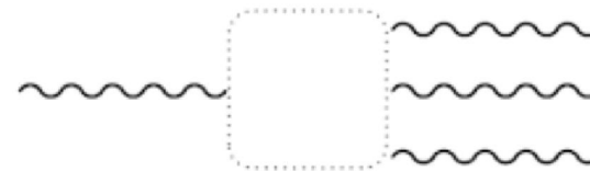
Figure 5. Four-wave mixing. It represents the combination of four electromagnetic waves. These effects are allowed in vacuum.
