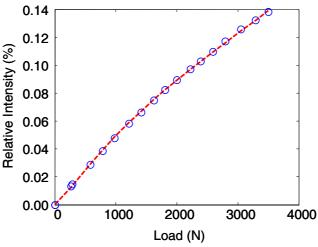
Figure 3: Relative light intensity (circles) transmitted through the interface as a function of the applied load for rough (500nm RMS) samples. Measurements (circles) are in excellent agreement with values (dashed line) calculated using equations 4 and 5.
