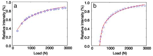
Figure 2: Relative light intensity transmitted through the interface as a function of the applied load for smooth samples. Measured values (circles) are compared to values calculated using equations 4 and 5 (dashed line). (a) PMMA on PMMA (b) PMMA on Glass In both (a) and (b) both sides of the interface had a 50nm rms roughness.
