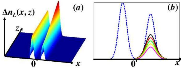
Fig. 1. (a) Linear refractive index profile. (b) Transverse profile of the refractive index at the input face [blue dashed line], along with the intensity profiles of five mutually-incoherent waves (solid lines), at the input face of the directional coupler. Each wave has different initial intensity. All the waves are launched into the right waveguide, where they form the incoherent beam.
