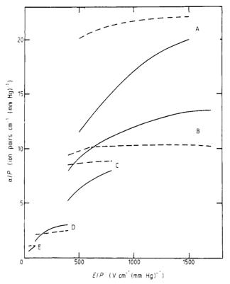
Figure 1. First Townsend ionisation coefficient. A, Hg; B, Ar; C, N<sub>2</sub>; D, Ne; E, He. Broken curves, calculations; full curves, experimental results.
